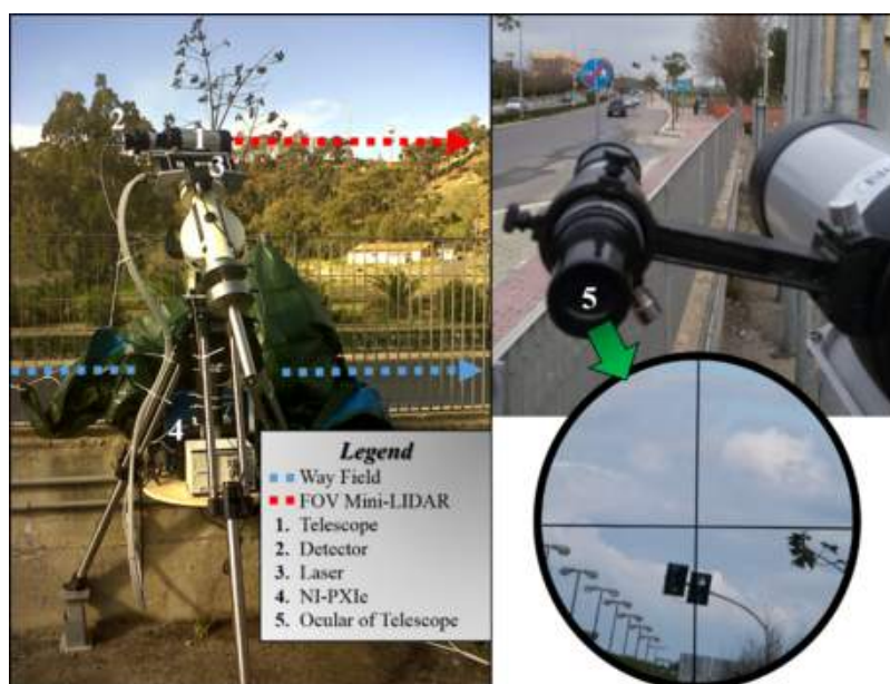
Figure 2. COLI experimental set-up during the experimental campaign of Crotona, February 2015. In the figure the laser source and the receiver are at the same location and the system is biaxial.
